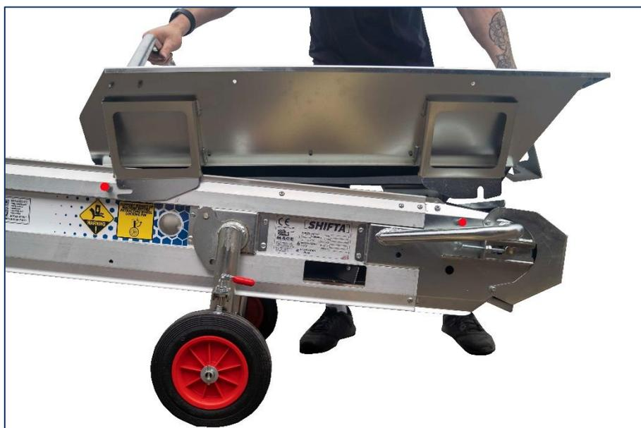
**5.** Once machine is in place. Plug in power supply at the base of the conveyor and start pre-operation checks
