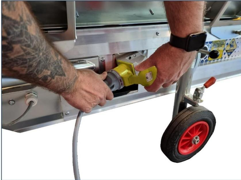
Then using the power linking lead supplied, plug the linking lead into the power output socket on the end of the conveyor then into the power input socket of the next conveyor. **Up to 5 conveyors can be powered off a single 5kVA supply.**
