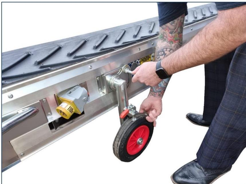
**3.** Manoeuvre the conveyor into position using correct manual handling techniques. Utilise the handles at the top and base of the conveyor to maximise grip when moving. When in position locate the conveyor onto the supplied trestle. This will allow the transported material to drop directly into the next conveyors hopper. Ensure that the brakes are applied at this point.
